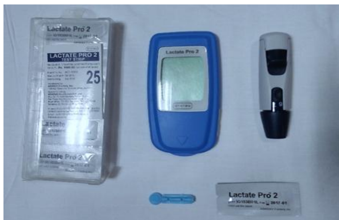
Fig 1: Lactate analyser with lancet, needle and testing strips
